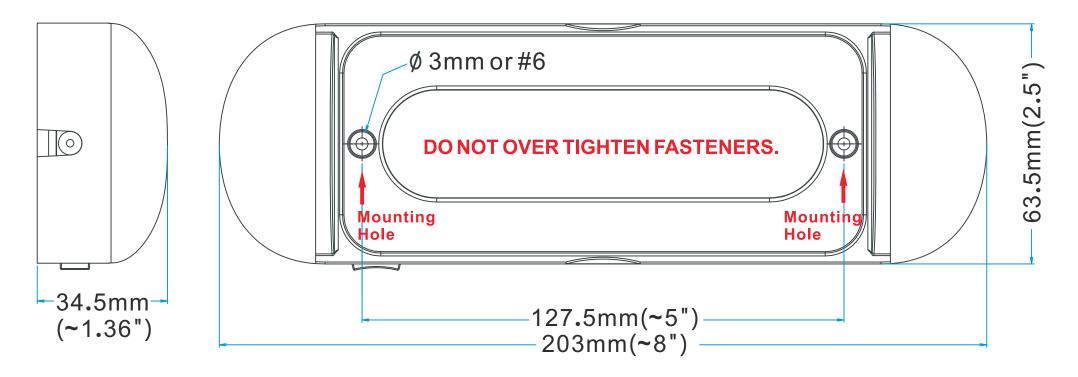
Use this template as your guide to find a suitable mounting location for this light. Then drill two small holes as marked on this template, wire the light, remove the front cover and install light with fasteners provided.
